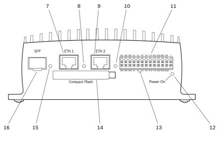
7 ETH 1 RJ45 socket for connecting to an Ethernet LAN (local network), 10/100 MBit Base-T
